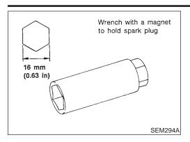
4. Remove spark plugs with suitable spark plug wrench. **Spark plug (Platinum-tipped type):**
