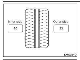
Indicated unbalance value  $\times$  1.6 = balance weight to be installed
